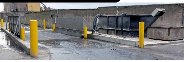
Tecnoter E series wheel washers are powerful closed-loop mobile systems, consisting of one or more washing lines served by accumulation and clarification units with integrated sludge extractor.
